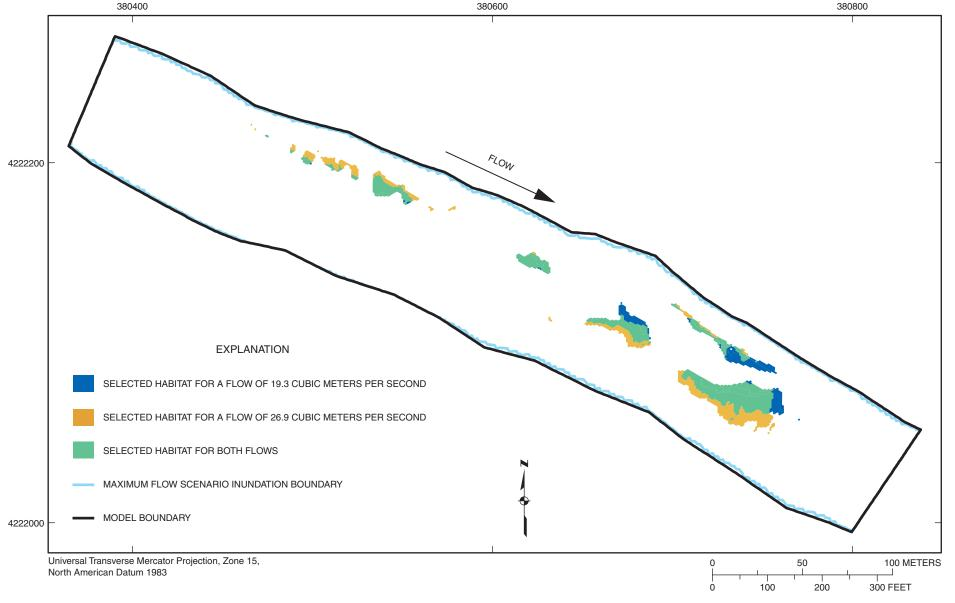
Figure 5-15. Selected habitat area distribution for habitat categories 4, 5 combined (slenderhead darter) at flows of 19.3 and 26.9 cubic meters per second at Marais des Cygnes River site MDC3.
